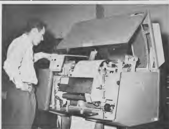
THE ASTONISHING IBM 1403 printer can actually print up to 600 lines a minute. Each line has 132 characters. The high quality printing is accomplished by engraved type suspended on a high-speed revolving chain. E SORPRESENTE impresor IBM 1403 ta realidad por druk te 600 linea pa minuut. Cada linea tin 132 letter di cifra. E drukmento di alta calidad ta worde haci door di letter grabá cu ta pansa ariba un cadena giratorio di alta velocidad.
